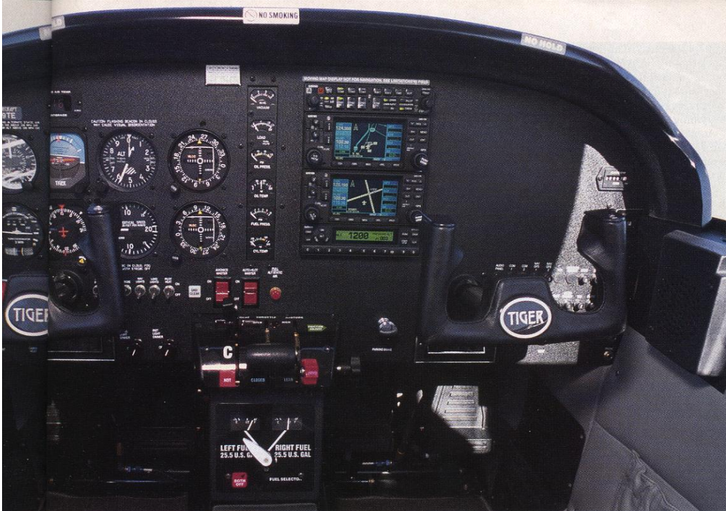
A new panel (above) incorporates Garmin avionics and an S-Tec autopilot. No rivets mar the sleek wing (above left) or control surfaces.
