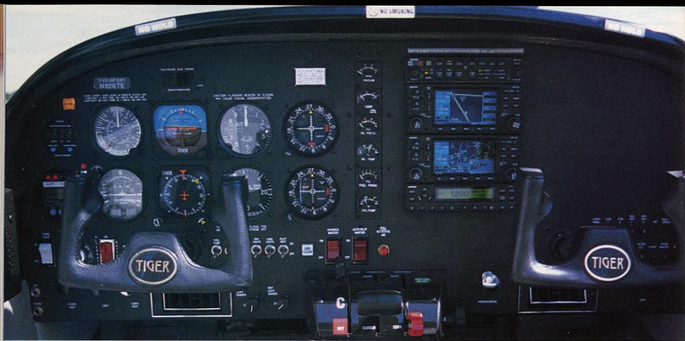
The panel of the Tiger is all new. With twin Garmin 430s, leather-wrapped yokes and vertically aligned engine gauges, the look of the Tiger is modern and clean.
