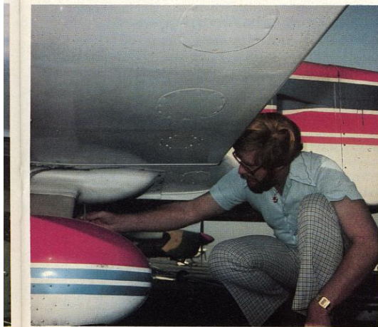
Four fuel sump drains on the Tiger are checked with a special fuel sampler cup.
