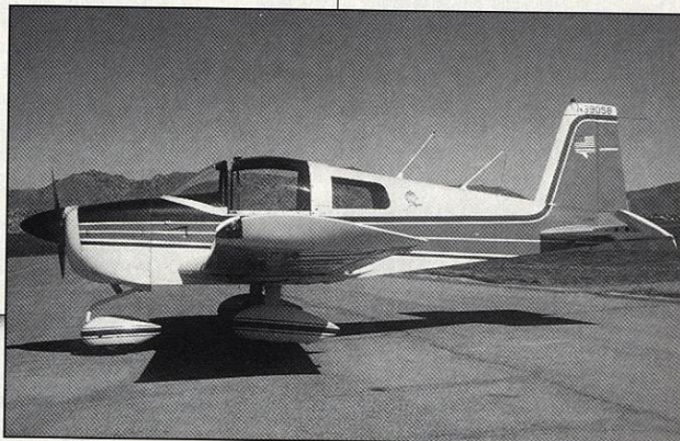
A profile view of the Lynx shows its rather boxy lines; it was cheap and easy to build, but aerodynamically inefficient. On the other hand, the bonded airframe, honeycomb-sandwich cabin and aluminum-tube wing spars make it incredibly strong.
