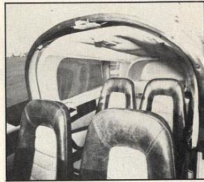
The rear seat cushions can be removed and the seat back folded down to provide a large area for hauling bulky items or even sleeping in the plane
