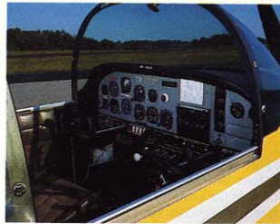
The Tr2's instrument panel space in the 40-inch wide cockpit is adequate for most VFR and IFR requirements.
