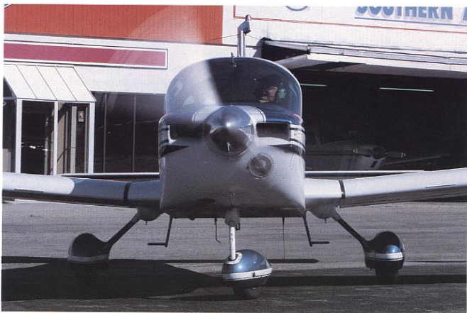
The Tiger's nosegear with its shopping cart-like castering wheel contributes to higher-than-average brake pad wear—a consequence of the steer-by-brakes system.
